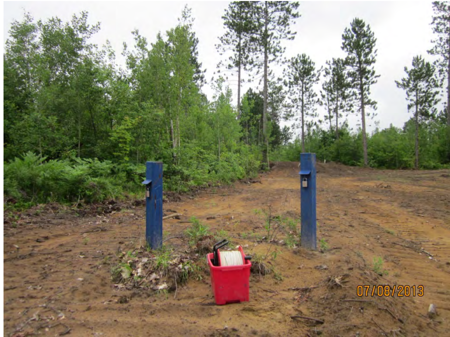
Photo 1 Groundwater monitoring wells BH1-I and BH1-II, July 2013
