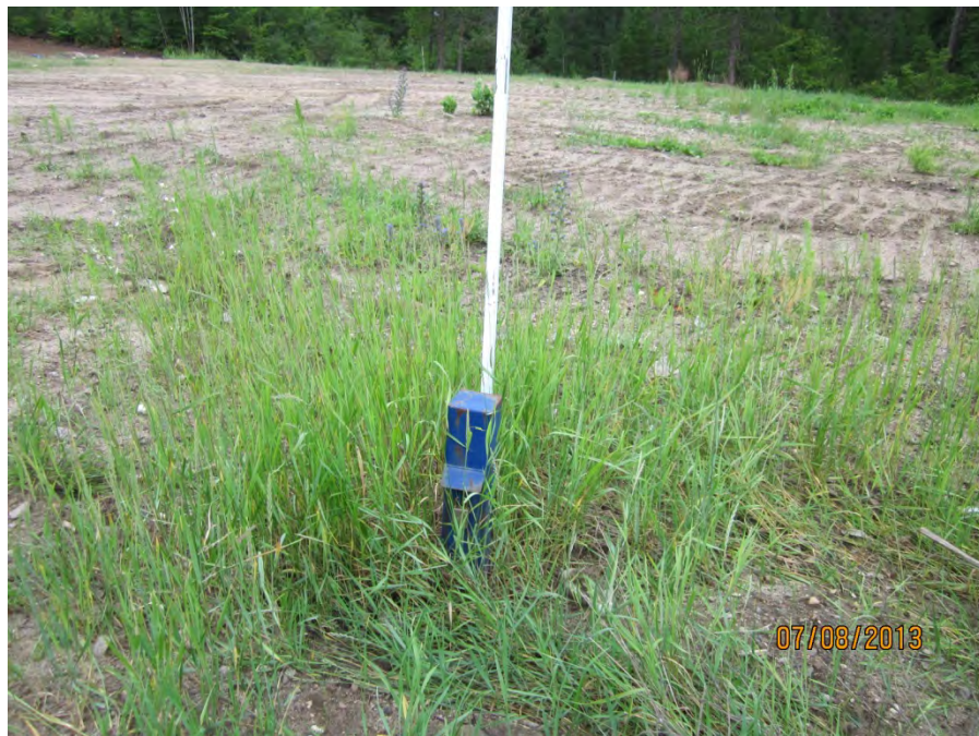
Photo 6 Groundwater monitoring wells BH5, July 2013
